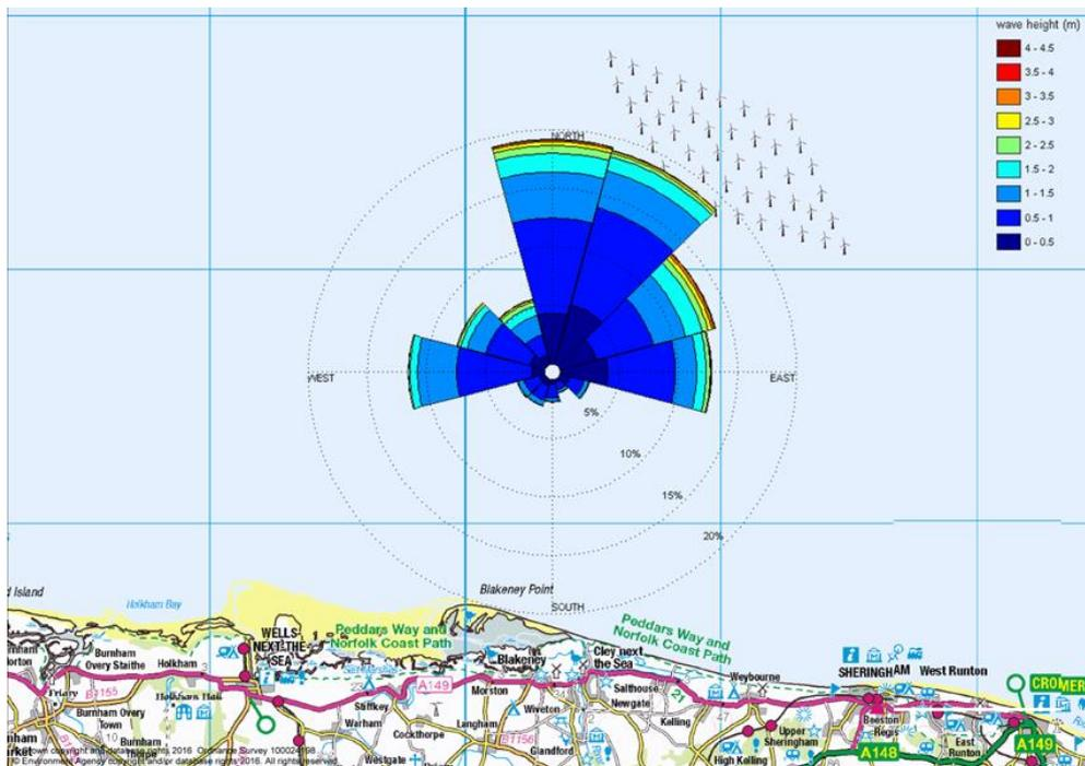
Figure 3: Wave rose plot for Blakeney Overfalls DWR off the Norfolk coast, for waves recorded from October 2011 to August 2015.
