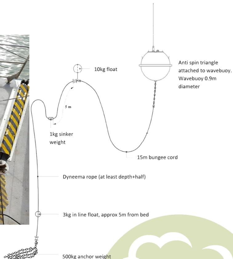
Figure 1: Wavebuoy and mooring on deck ready for deployment (left). Diagram of a wave buoy shallow water mooring (right) (image: Gardline Environmental)
