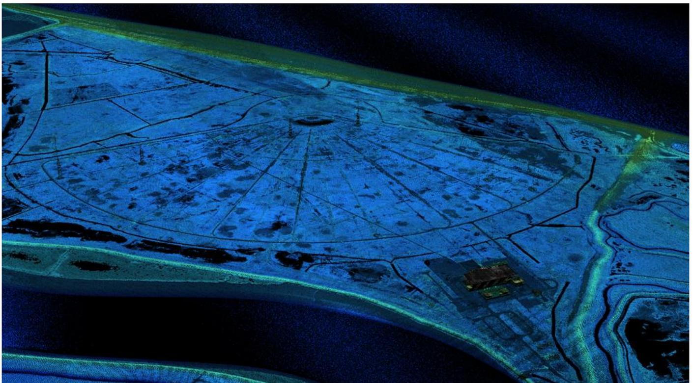
Figure 3: The point cloud output from a LIDAR survey over the Cobra Mist site at Orford Ness, Suffolk.
