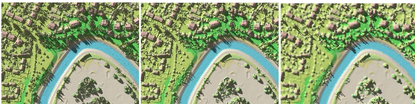
Figure 5: Examples of LIDAR resolutions at: 25 cm (left), 1 m (middle) and 2 m resolution (right)..
