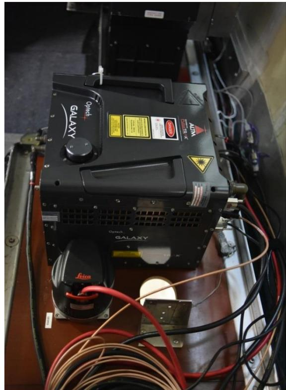
Figure 1: LIDAR sensor mounted inside the aircraft
