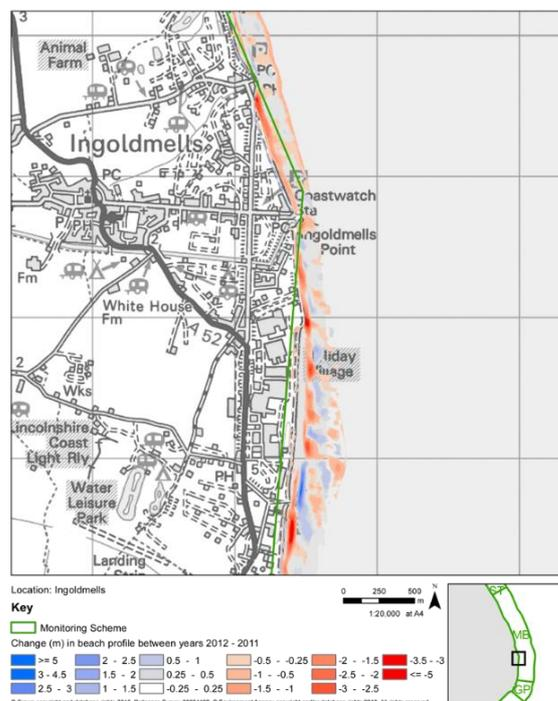
Figure 6: Elevation change analysis and difference model of the beach at Ingoldmells, Lincolnshire
